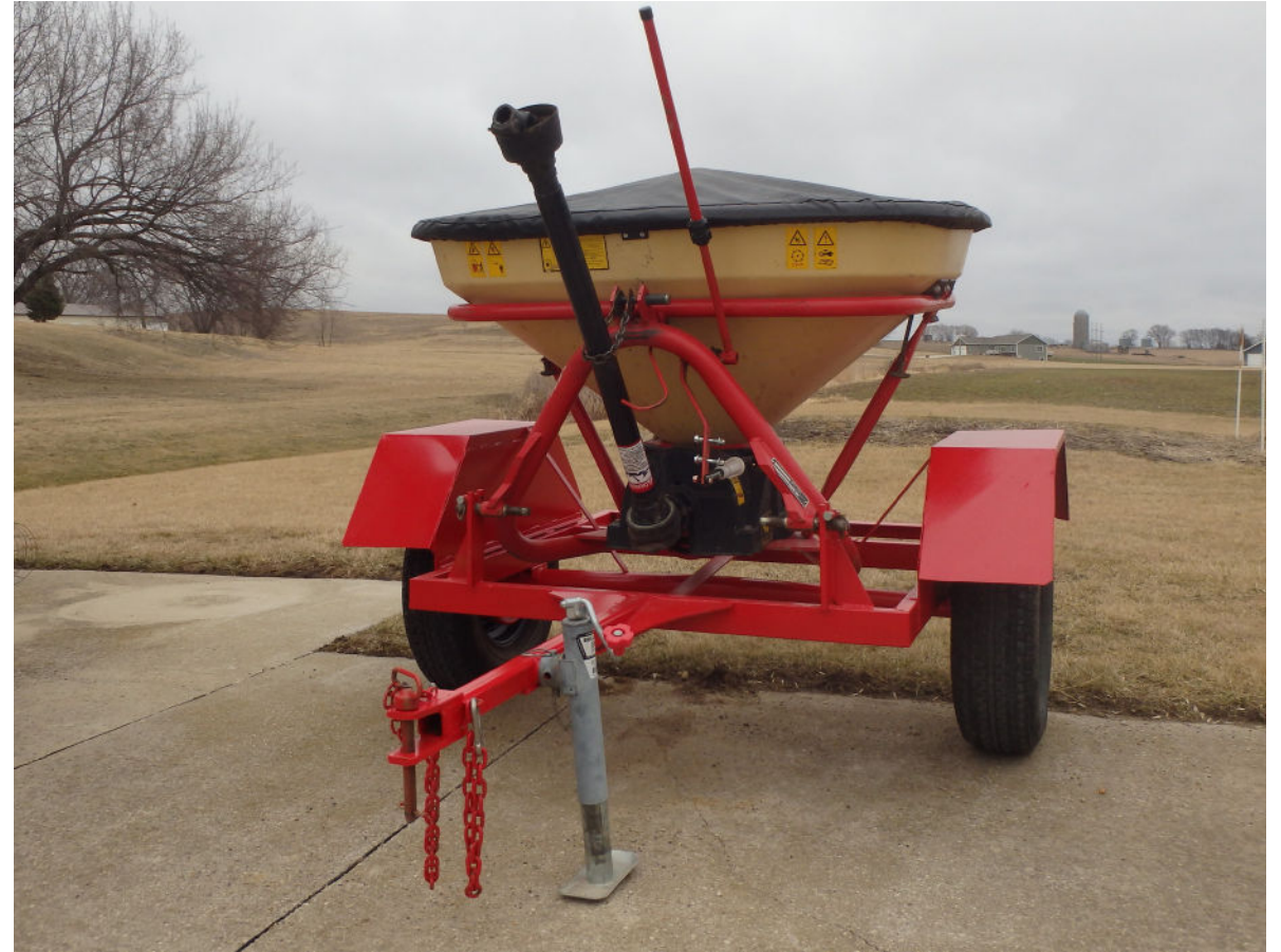
The District also has a Vicon broadcast seeder that is available to rent to producers who wish to do their own seeding. It fits on a 3-point hitch and has a 15- foot spread.
